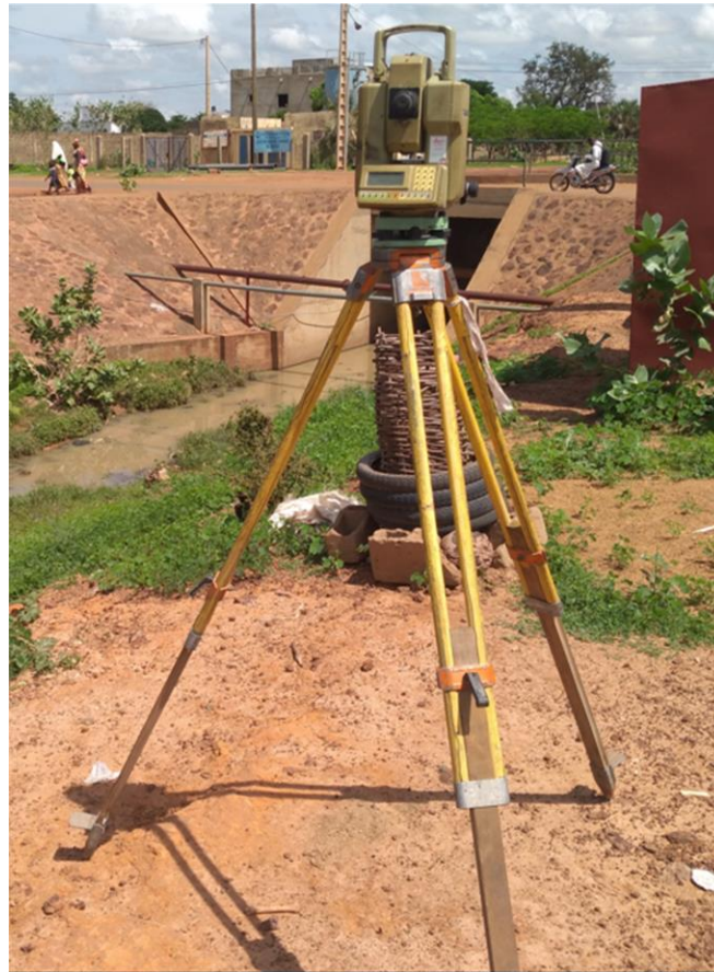
Figure 5 Total station Leica on the terminal base
